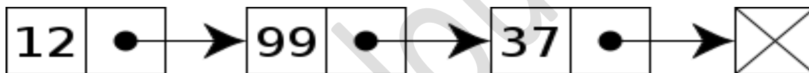
A linked list whose nodes contain two fields: an integer value and a link to the next node
